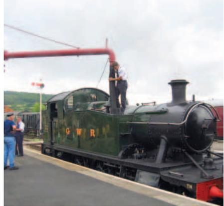
A steam train derives its power from an engine which produces steam in a boiler, usually fuelled by coal. As the fuel heats the water in the boiler, steam is generated and that is used to drive the locomotive, as well as working the whistle, brakes, pumps and heating throughout the carriages.
